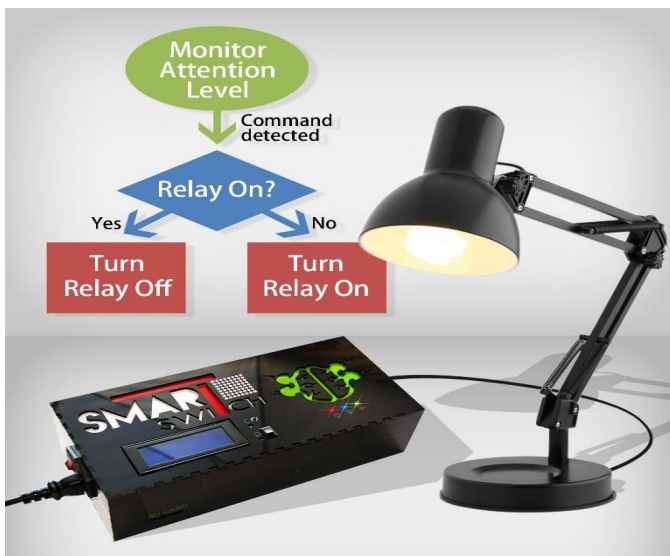
Fig. 8 - The developed system used as a control for a desk lamp.
